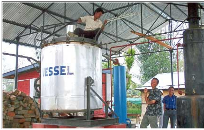
A distillation plant for citronella/lemongrass/patchouli set up by Mr Bitu Luhu at Chumukedima, Dimapur
