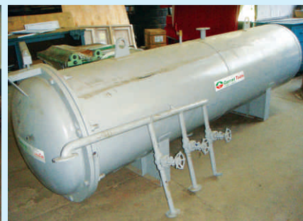
Bamboo Treatment Plant
