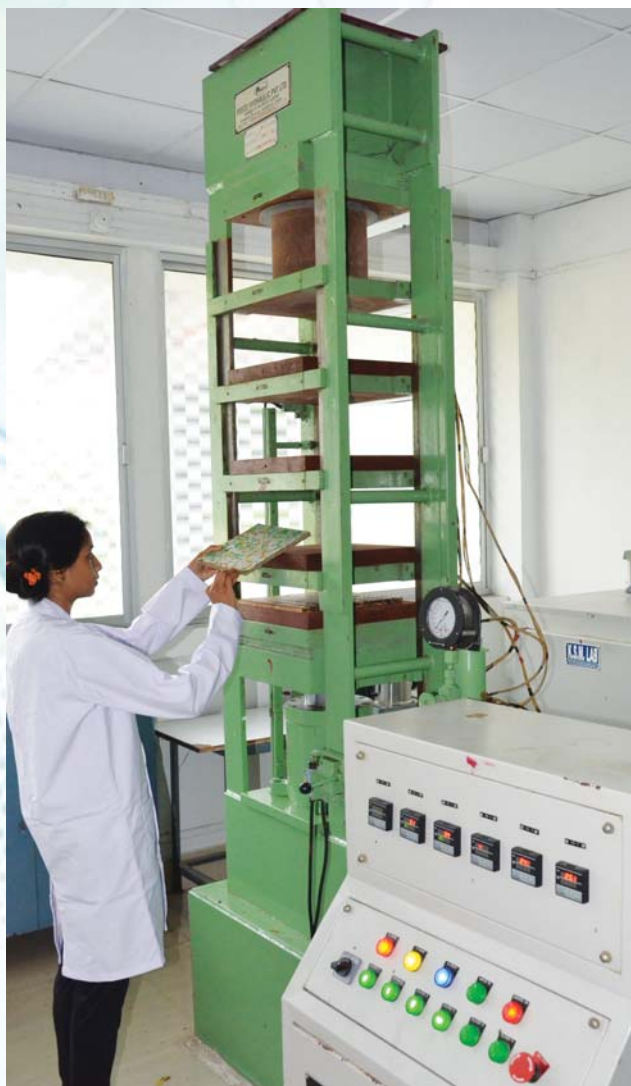
Fig: Multi Layered Hydraulic Hot Press For Making Composite Board
