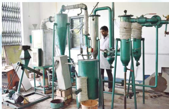
Fig: Integrated Coal-Based Gasifier System
