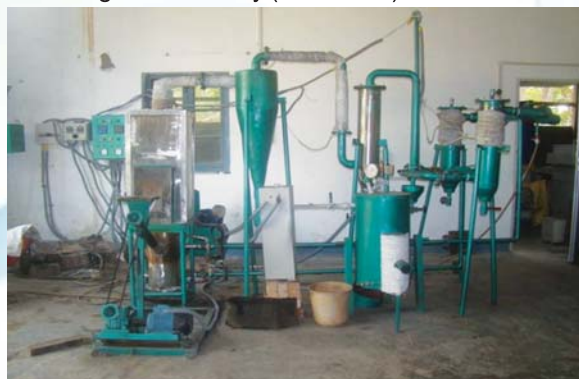
Fig: Integrated coal-based Gasifier system
