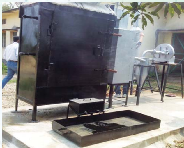
Fig: Prototype for removal of solid deposits from strainer installed at OIL PS-3
