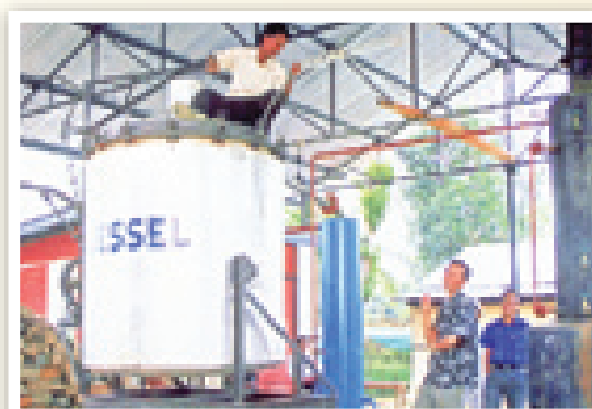
Commercial aromatic oil extraction plant setup by Mr Bito Luhu of Chumukedima, Dimapur, Nagaland which is manufacturing various aromatic oils like citronella, lemon grass, patchuli etc.
